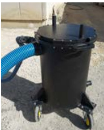
Portable filtration device – 50 litres/minute using a transfer pump
